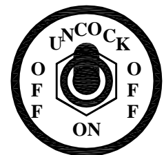
UNCOCK position: To unarm the machine.
