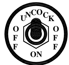
UNCOCK position: To unarm the machine.
